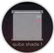
**Battery level displayed in red** indicates the shade motor battery has reached critical level. At this point, the shade motor is not expected to perform at its peak status.
