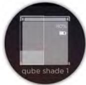
**Battery level displayed in white** indicates the shade motor battery is above the threshold. The battery level does not show if at or above the threshold warning.
