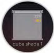
**Battery level displayed in yellow** indicates the shade motor battery level has fallen into warning level. As shown, the threshold can be edited in Design Center. Additionally, at this level, shade motor performance will begin to drop.
